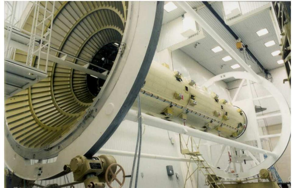
**It is designed for installation of 12 spacecraft. It is manufactured from high-strength aluminum alloy and equipped with ventilation system and separation system**
