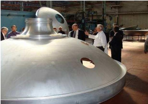
**Oxidizer Tank Bottom Dome**
