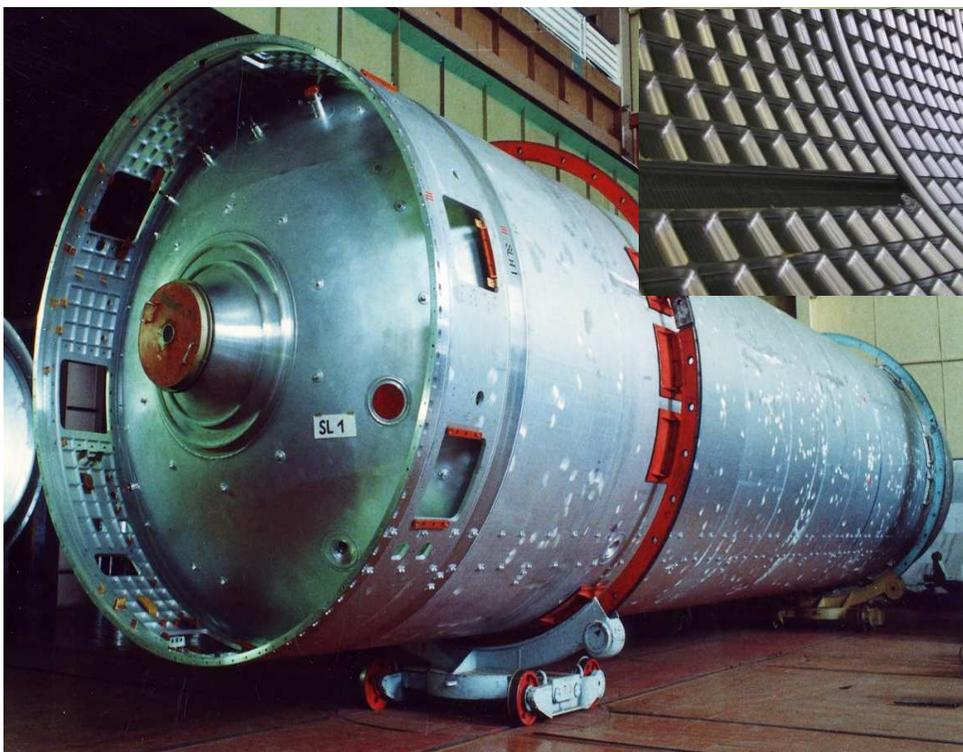
**It is manufactured from aluminum alloy and has waffle structure.**
