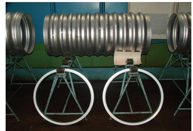
**Fuel Tank Tunnel Pipeline (for Oxidizer Feedline)**
