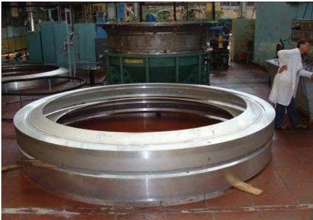
**Bulkhead for Fuel Tank Bottom Dome**
