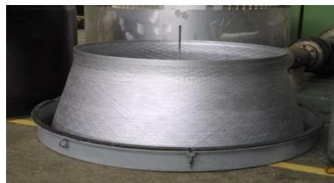
Nozzle extension for Solid-propellant rocket engine
