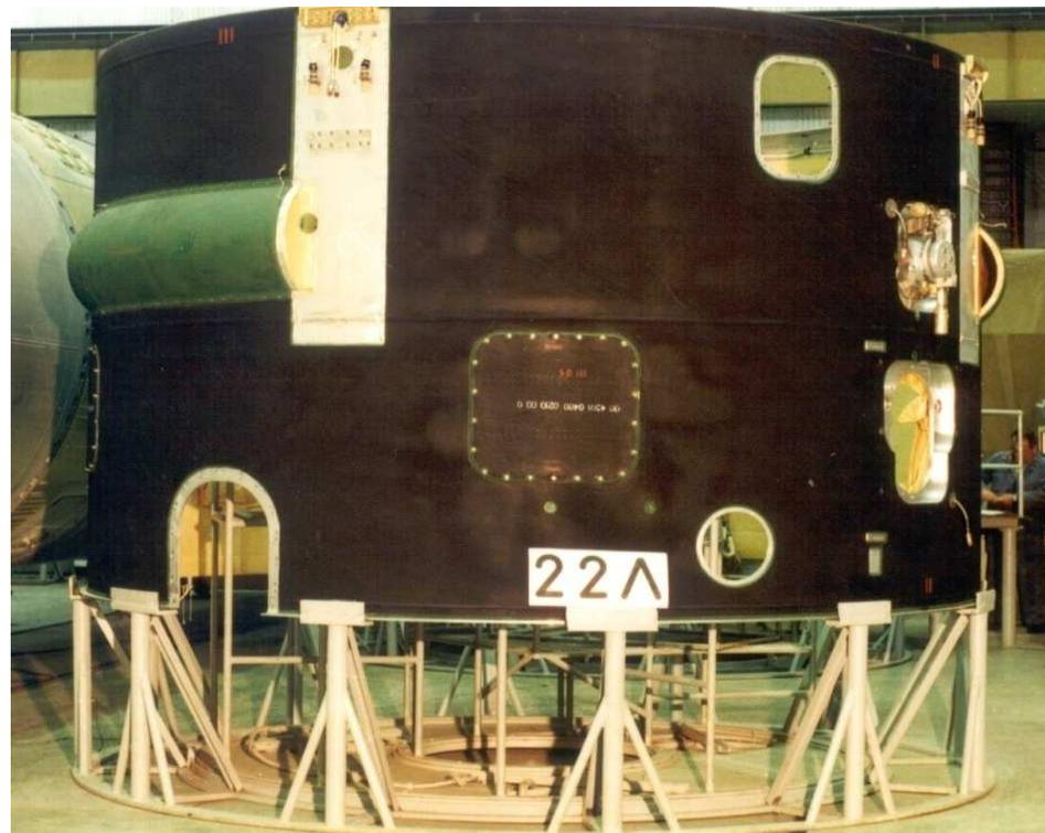
**It is manufactured from aluminum alloy and covered by high-efficient heat-protection material**
