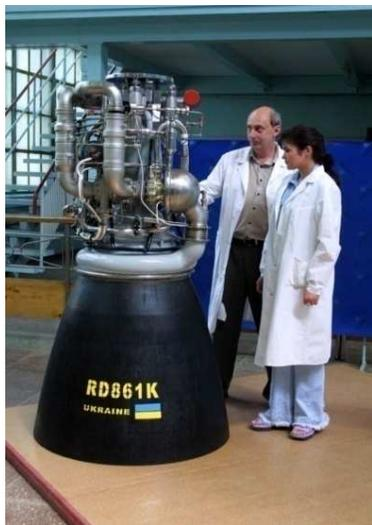
Liquid-propellant rocket engine with uncooled nozzle extension made of carbon-carbon
